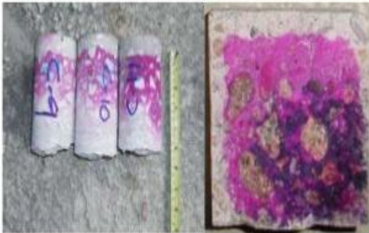
Test Cylinder After Phenolphthalein Indicator Applied.
