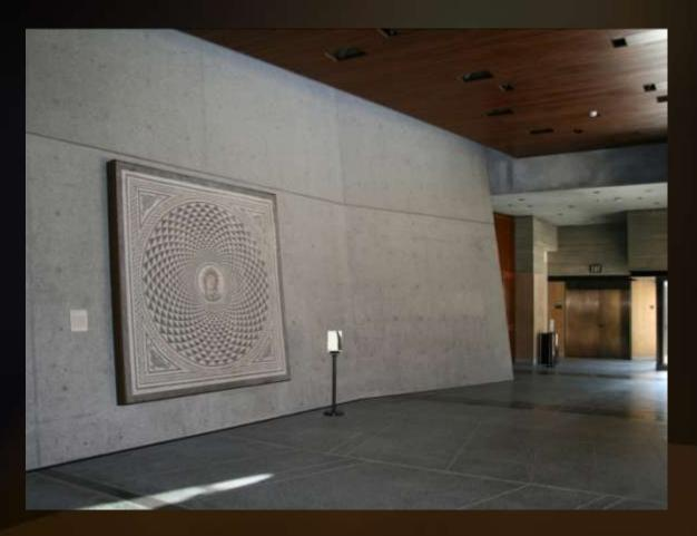
Formed, textured and sandblasted concrete Interior and exterior walls, floors and paving
