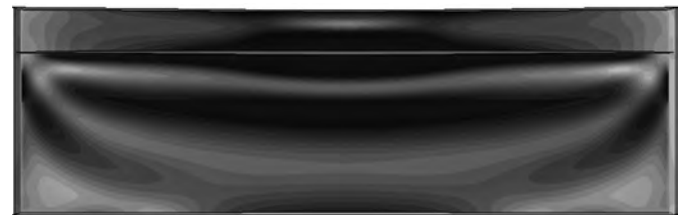
Web folding of both loaded panels
